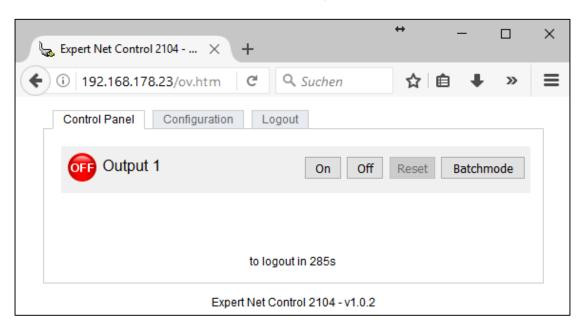
12. **To turn on the mount:** Press On - wait for three seconds - press Off. The mount will boot, which is indicated in the keypad display by *Connecting* .... Previously you must have defined that the Virtual Keypad should connect after startup (**AutoConnect**).
