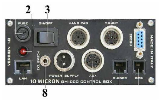
The *expert net control 2104* switching module must be operated as a rocker switch. It must close the contact for one to three seconds, but not continuously: Switch on – wait for 3s – switch off. The mount is now switched on. Same procedure for switching off the mount: Switch on – wait for 3s – switch off.
