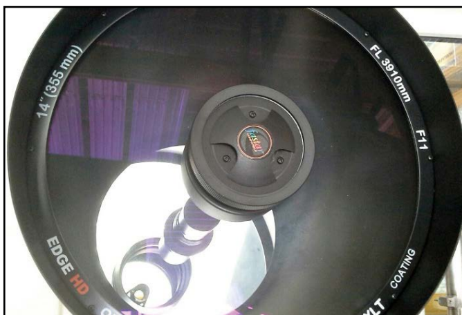
C14 EdgeHD with fogged Schmidt plate (in the right third, diagonal)
