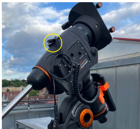
Strain relief for the power cable, which is tied up to the mount with Velcro tape. This also prevents contact losses due to loose contacts.
