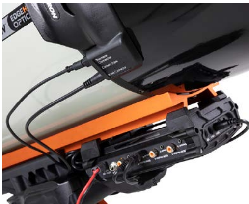
Short cables on a fixed distributor, here the Celestron dew control with integrated power distribution for other devices.
