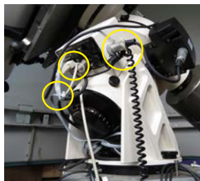
Secured cabling on an AstroPhysics mount. Center: Detailed view of the combined RS-232, guiding and power cables as well as the strain relief on the plug of the hand controller. Right: Detailed view of the strain relief of the very heavy spiral cable of the hand controller at the plug of the RA motor cable.
