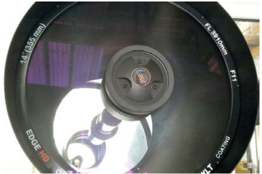
C14 EdgeHD with foggy Schmidt plate (in the right third, diagonally)
