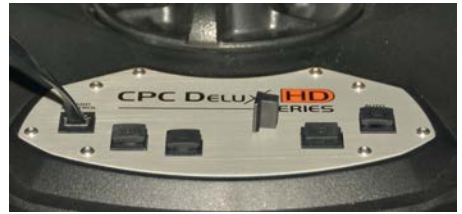
Cover caps prevent moisture from getting into unused sockets or cables from being connected incorrectly and causing short circuits.
