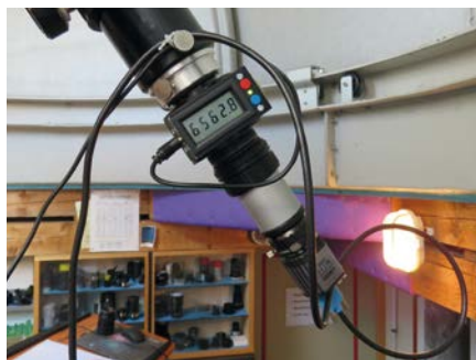
Cable protection on an H-alpha filter: Looped, strain-relieved cables for USB 3.0 and power supply, attached to the clamping screw of the focuser
