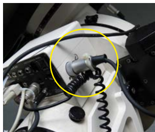
Secured cabling on an AstroPhysics mount. Center: Detailed view of the combined RS-232, guiding and power cables as well as the strain relief on the plug of the hand controller. Right: Detailed view of the strain relief of the very heavy spiral cable of the hand controller at the plug of the RA motor cable.
