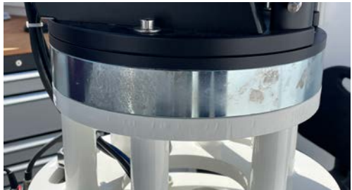
Normal ageing: A galvanized stainless steel flange after one year in a ventilated, non-air-conditioned hinged roof shed. The material eventually becomes completely matt due to environmental influences, but does not rust.
